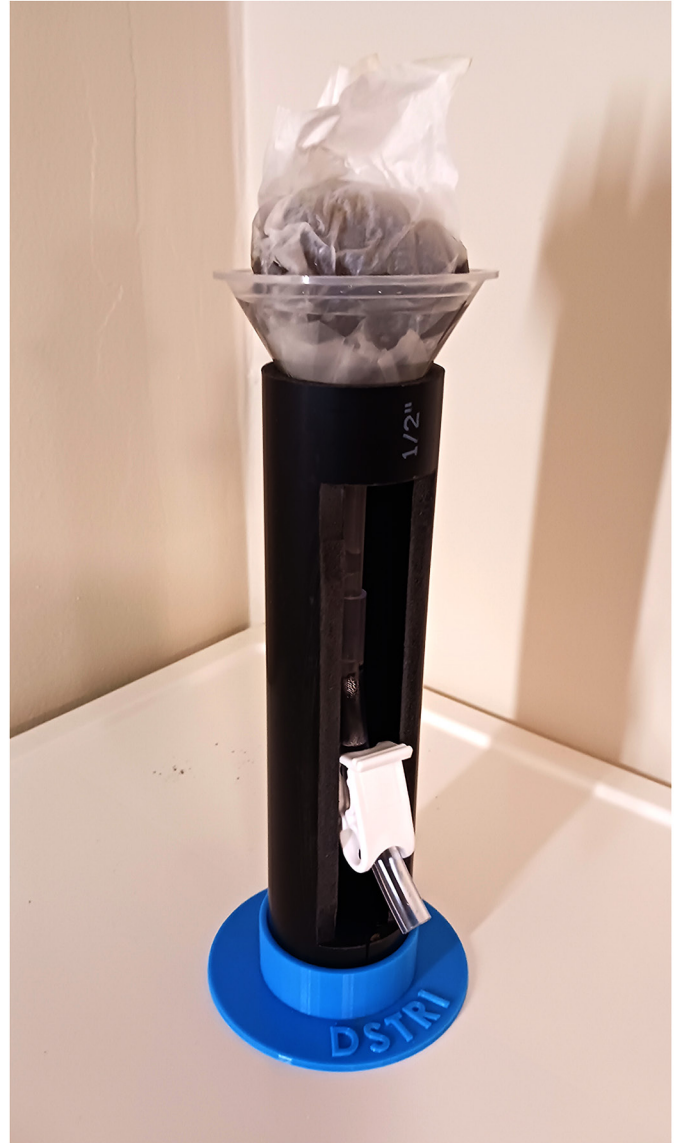
Figure 8: Baermann funnel set up for live nematode extraction from E. annectens femur fragments.
